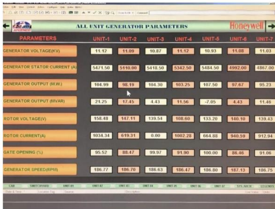
Fig 7 SCADA Based Real-Time Monitoring of Generator Parameters For Multiple Units At the bottom, there are status indicators and alarms showing system conditions like supply failures, disturbances, and faults. Green indicators represent normal conditions, while red signals warnings or failures. Overall, this interface helps operators safely control and monitor power generation systems in real time.
