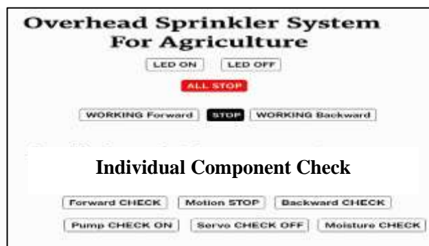
Fig. No.5 Interface of Controller
