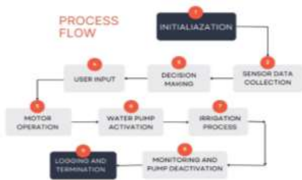
Fig. No. 4 Process Flow Diagram of irrigation system
