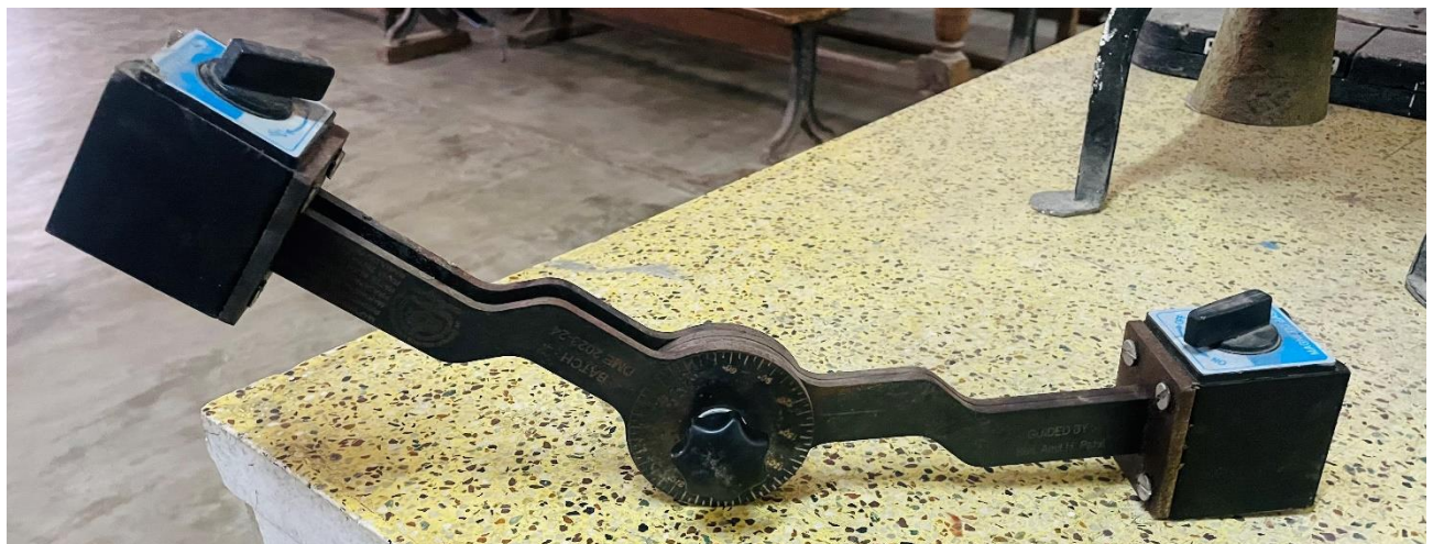
Fig. 3.2 Original Multi Angle Magnetic Welding Fixture
