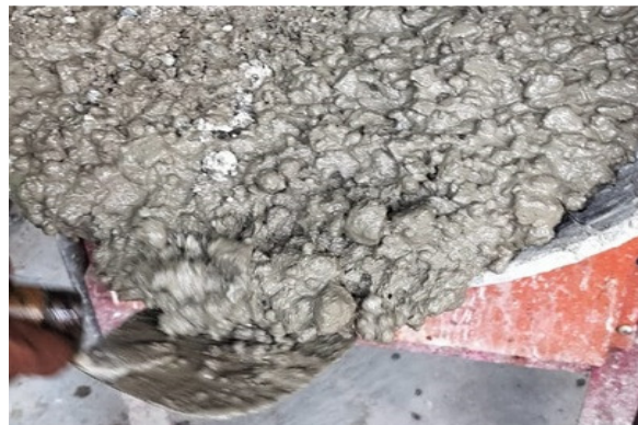
Figure 5: Geopolymer concrete fresh state
