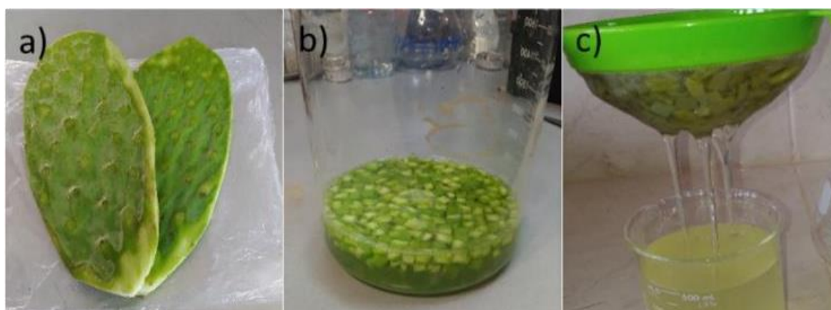
Fig2. a) Fresh cactus leaves, b) Prickly pear cactus mixed with water c) Filtration process of Nopal mucilage[15]
