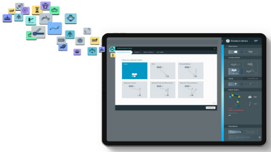
Figure 3: The GUI used for FRANKA EMIKA products that utilizes a workflow-based robot programming approach [EMI].
