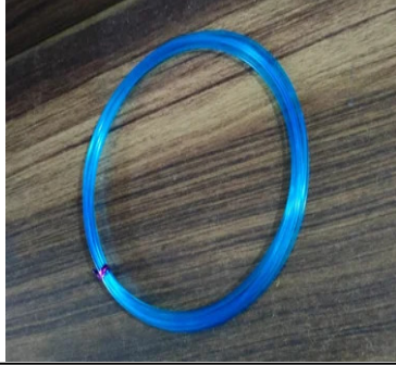
Fig 7. Quality smooth 3D filament hollow c/s from recycled PET plastic waste.
