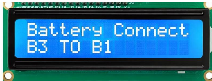
Figure 6. Battery is connected between BP3 to BP1 for Active cell Balancing
