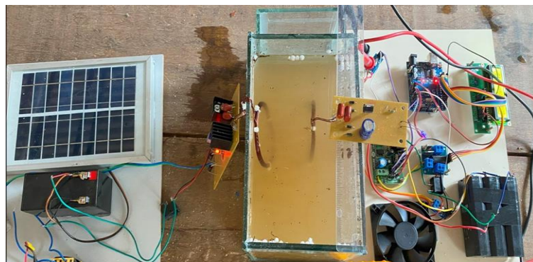
Fig 9. Experimental Setup of UWPT for Normal Water
