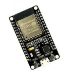
ESP32 based boards come in a variety of shapes and sizes and pinout of each board is different to other. Also, not all pins of the ESP32 Microcontroller SoC will be available on a development board as some pins might be permanently tied to a dedicated function.
