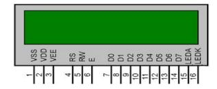
It is called Liquid Crystal Display. We are going to use 16x2 characters LCD. This will be connected to microcontroller. The job of LCD will be to display all the system generated messages coming from the controller. LCD will provide interactive user interface. This unit requires +5VDC for it proper operation. This module is used for display the present status of the system.
