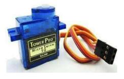
A servo motor is a type of motor that can rotate with great precision. Normally this type of motor consists of a control circuit that provides feedback on the current of position the motor shaft, this feedback allows the servo motors to rotate with great precision. If you want to rotate an object at some specific angles or distance, then you use a servo motor. It is just made up of a simple motor which runs through a servo mechanism. If motor is powered by
