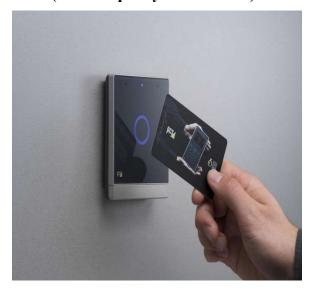
RFID (radio frequency identification) is a form of wireless communication that incorporates the use of electromagnetic or electrostatic coupling in the radio frequency portion of the electromagnetic spectrum to uniquely identify an object, animal or person. Use cases for RFID technology
