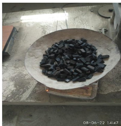
Figure 2: Rubber Aggregate after appropriate sizing
