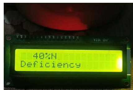
Figure 4. Display is showing status of Nitrogen on soil
