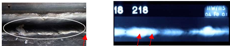
Figure 6. Undercut radiography film image
