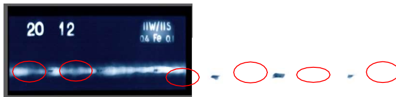
Figure25. Picture from radiography film and missing penetration cluster
