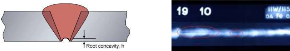
Figure 10. Concavity of the weld root and associated radiography film picture
