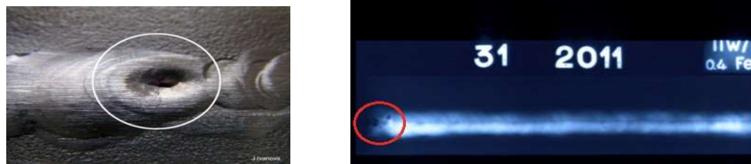
Figure 4. The accompanying radiography film image defines the end crater and star crack.
