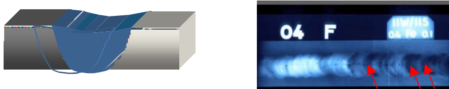
Figure 11. The image of under fill and its radiography film
