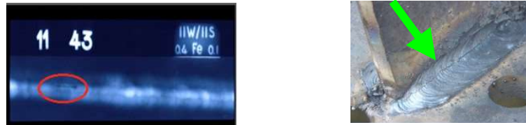
Figure2. Radiography film image of the longitudinal crack that has been shown in it and longitudinal crack
