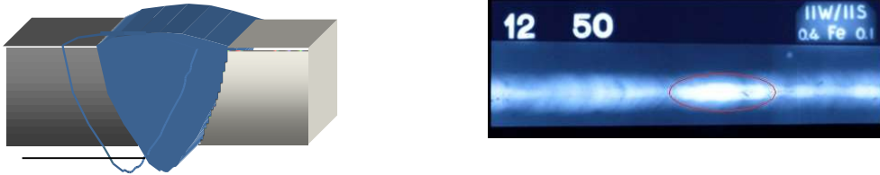
Figure 8. The radiography film image of excess penetration
