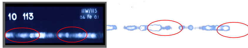
Figure 17. Image from radiography film and cluster of additional weld metal
