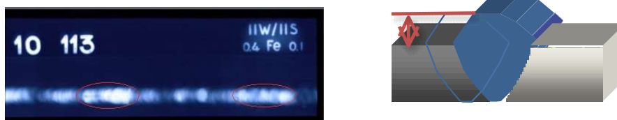
Figure 7. Overweld metal and the image of radiography film
