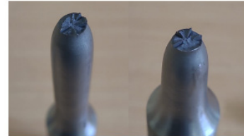
Figure - 4.4.1c - The fracture surface of SS410 after Tensile test
