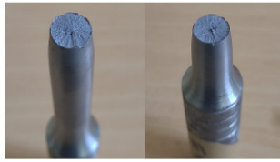
Figure - 4.4.2c - The fracture surface of EN-19 after Tensile test
