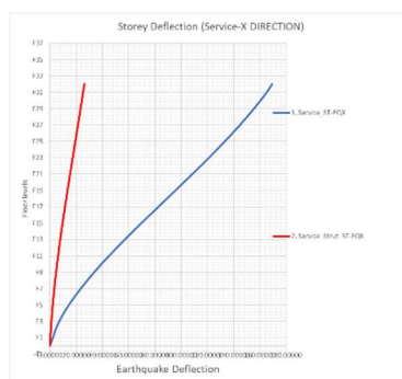
Figure 5.5 Earthquake story deflection in X- Direction
