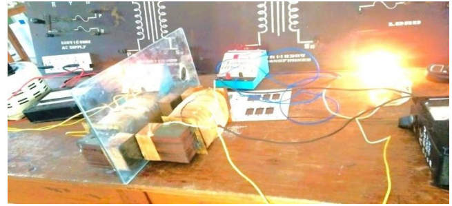
Fig 6 Experimental set up of WPT using silicon Steel using Glass as medium under load conduction
