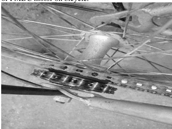
7: Sprockets for Motor and Pedal
