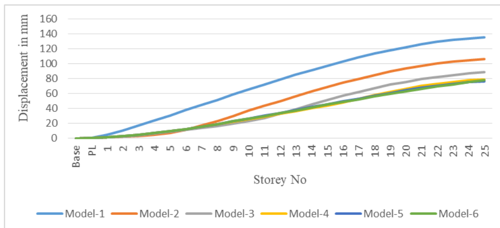
Graph -6.3: Displacement in mm of all models due to ESM along-Y direction
