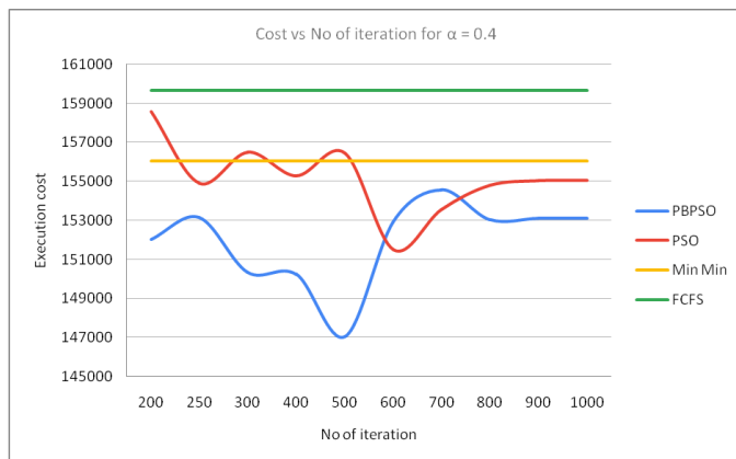
Fig 5. Cost for proposed PBPSO and existing algorithms for 200 to 1000 iterations at ( \alpha = 0.4 ).
