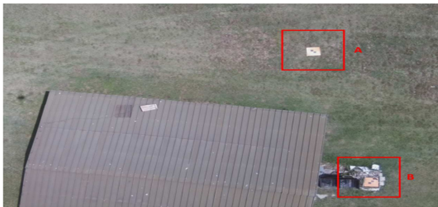
Figure 1: Marker placed on the ground (A) and a structure in elevation (B). (Marco Piras, Nives Grasso, Ansar Abdul Jabbar; 2017, Pg.291)
