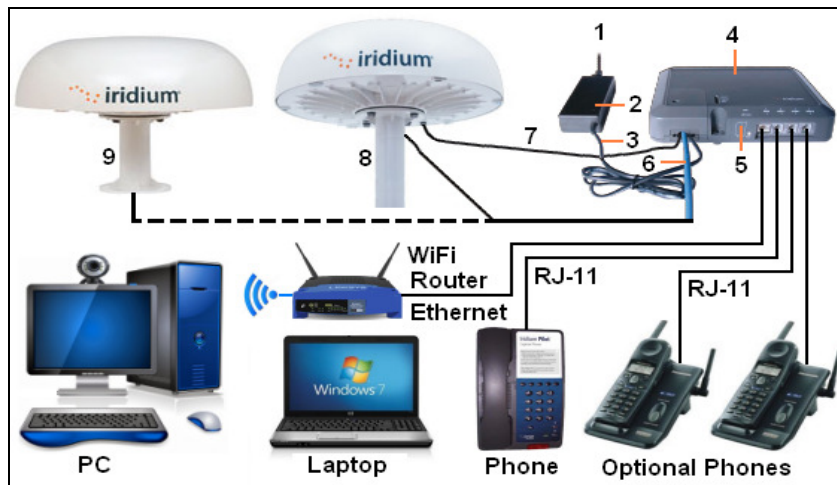
Figure 12. Iridium Pilot Broadband Station for Mobile and Fixed Applications – Source: Ilcev
