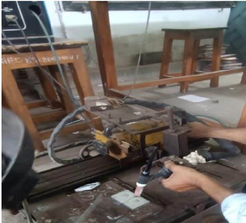
Figure 1: TIG welding machine setup
