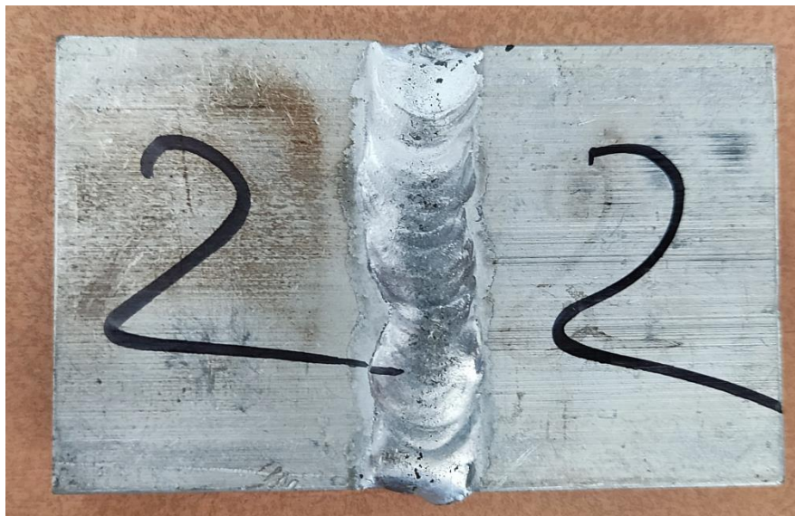
Figure 2: Typical TIG welded bead profile on Aluminium AA6063 alloy
