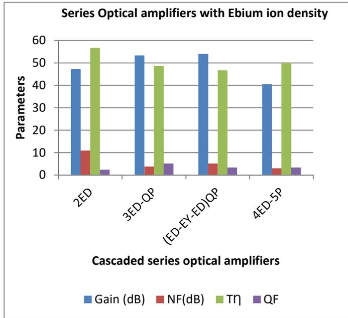
Fig. 7 . Parameters comparison of cascaded Series EDFA concerning Enhanced Erbium ion density
