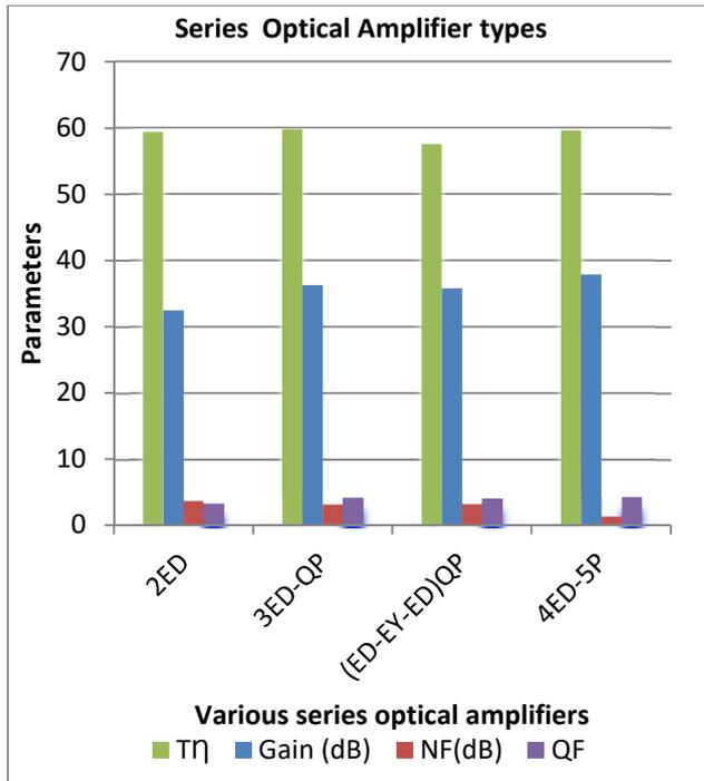
Fig. 6 . Parameters comparison of cascaded Series EDFA concerning Erbium ion density
