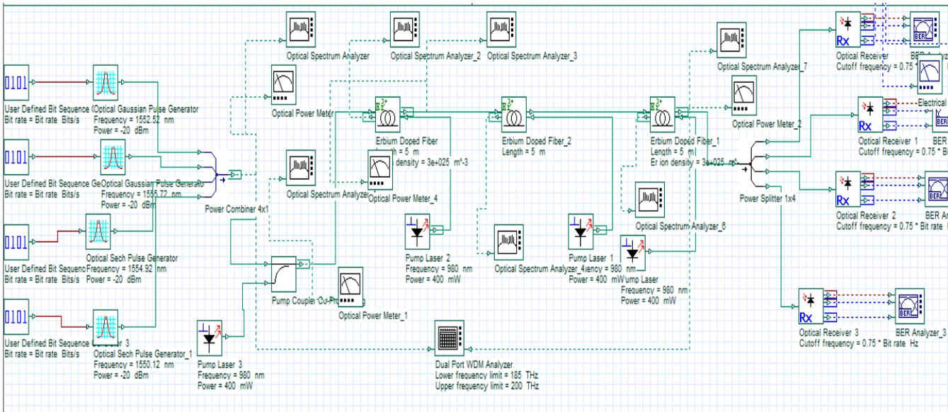
Fig. A-1. Three stages of series EDFA denoted as 3S-EDFA with quadruple pumping of Digital input data.
