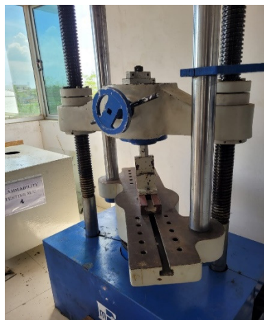
Fig.5 Interlaminar shear test Rig & Sample's
