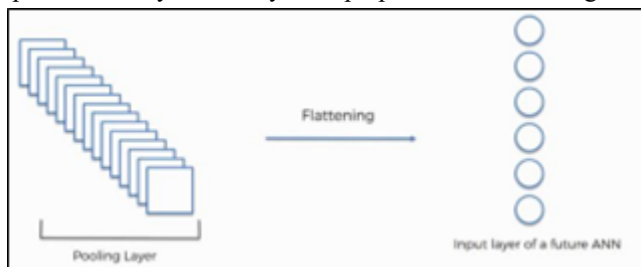
Fig 7: A diagram depicting Flattening of Pooled Feature Maps
