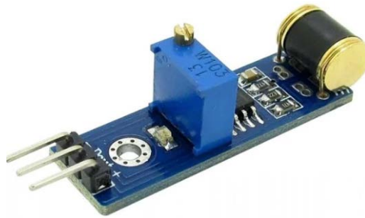
Fig -6: Vibration Sensor
