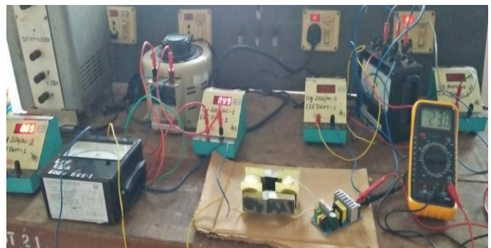
Fig 4: Experimental Setup for WPT System while Magnetizing and converting AC voltage to DC
