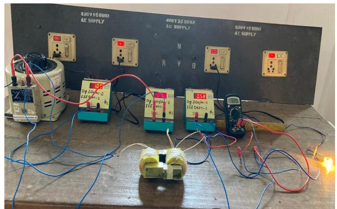
Fig 3 Experimental Setup for WPT System with litz wire on both side while Magnetizing
