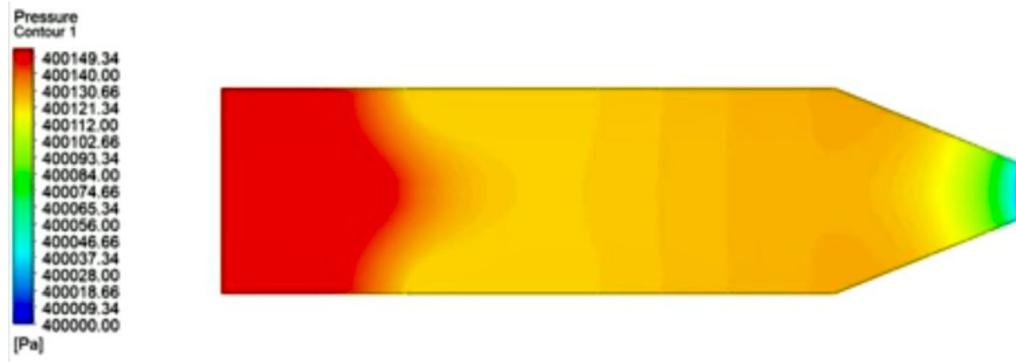
Figure 5. Pressure distribution in the gasifier
