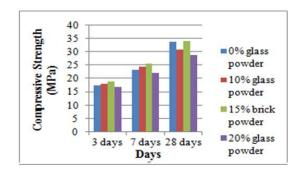
3.3 Comparison of compressive strength of M-25 mix for different percentage of Glass powder
