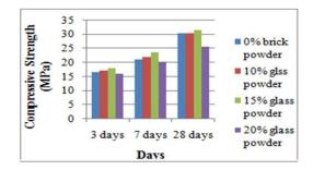
3.2 Comparison of compressive strength of M-20 mix for different percentage of Glass powder
